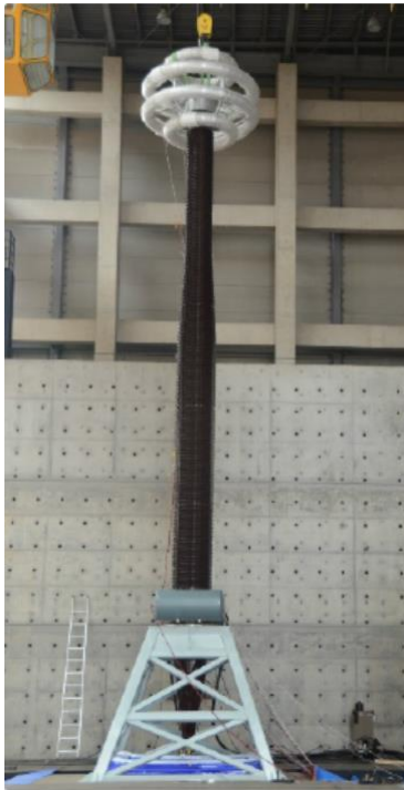
(a) Real insulator with varying cross-section
